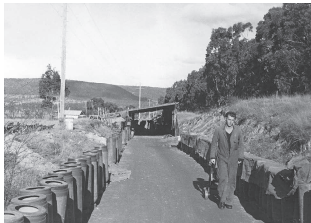
View of maintenance line just outside Marrangaroo tunnel with a temporary shelter at the rear. Mustard filled 250-lb light case bombs await venting on both sides of the road. The bombs were mid grey and stencilled with yellow paint for bomb identification. Brown detector paint was applied to detect gas leaks. The chemical warfare armourer pictured is Geoff Burn. Mid-1943.
